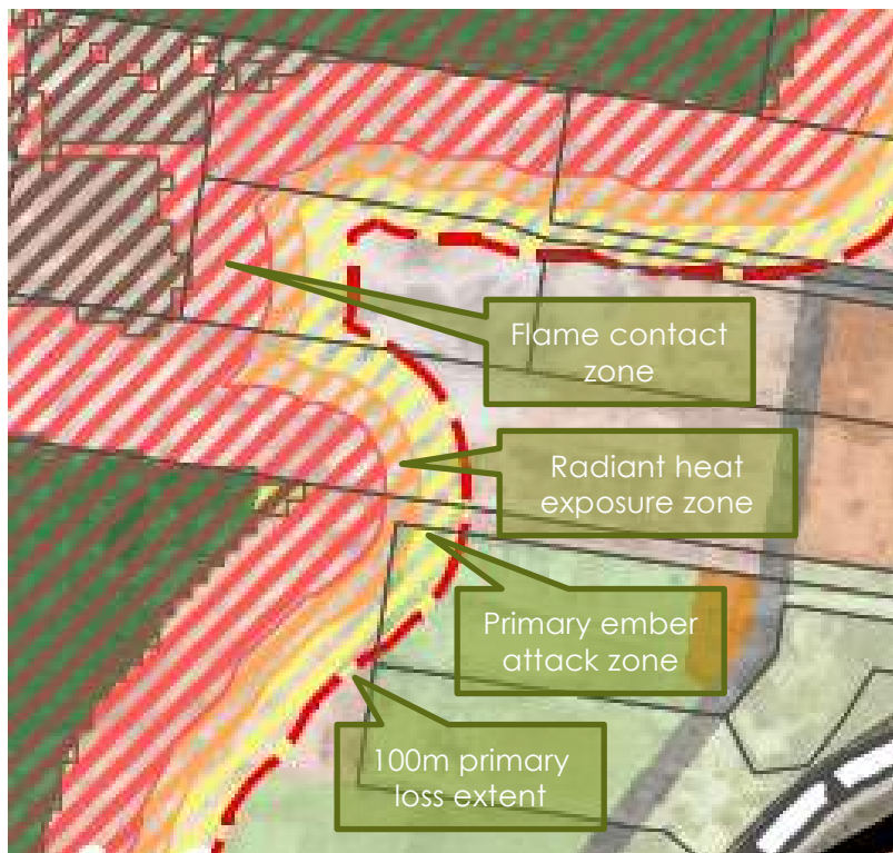
Figure 24 - Excerpt of proposed landscape risk exposure mapping, illustrating the 'primary loss extent'
