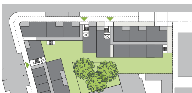
Figure 4F.5 Mixed use buildings may have a range of circulation spaces including multiple cores, gallery access and double-loaded corridors with cross-over apartments
