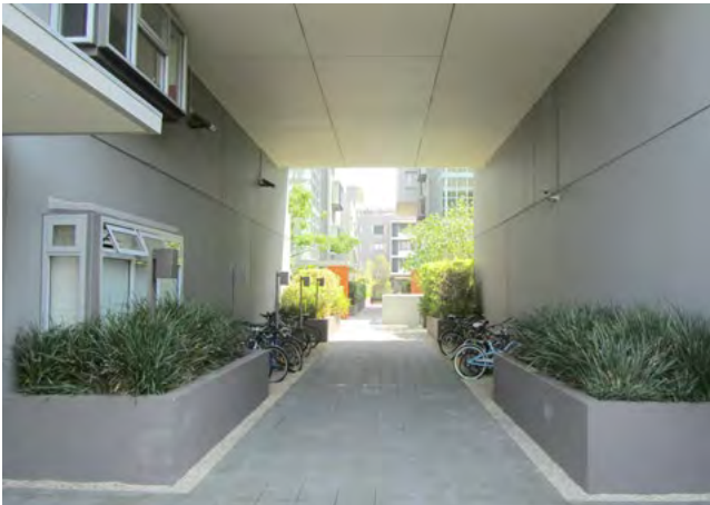
Figure 3G.5 Pedestrian through-site links need to be direct with clear sight lines to each end
