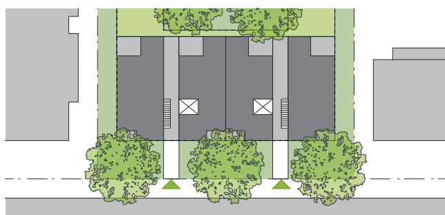
Figure 4F.4 Multiple cores improve natural cross ventilation and provide more entries along the street, increasing activity and passive surveillance
