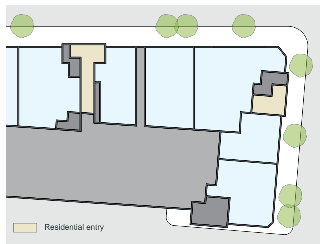
Figure 4S.3 Shop and office entries, service areas and loading zones in a mixed use development should be separate from lobby entries to residential apartments
