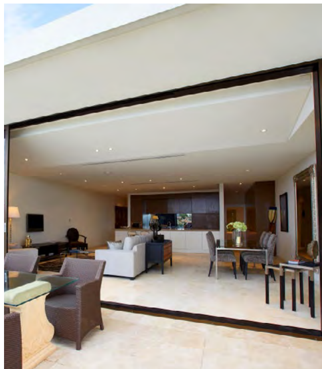
Figure 4D.2 For open plan layouts, combining the living room, dining room and kitchen, the maximum room depth is 8 metres from a window
