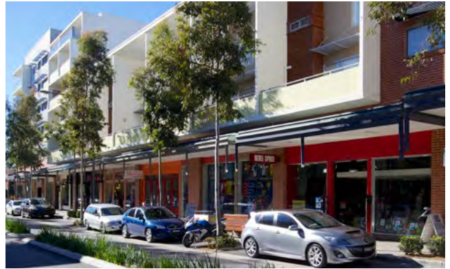
Figure 2G.1 For mixed use buildings with retail uses at the ground floor a zero setback is appropriate
