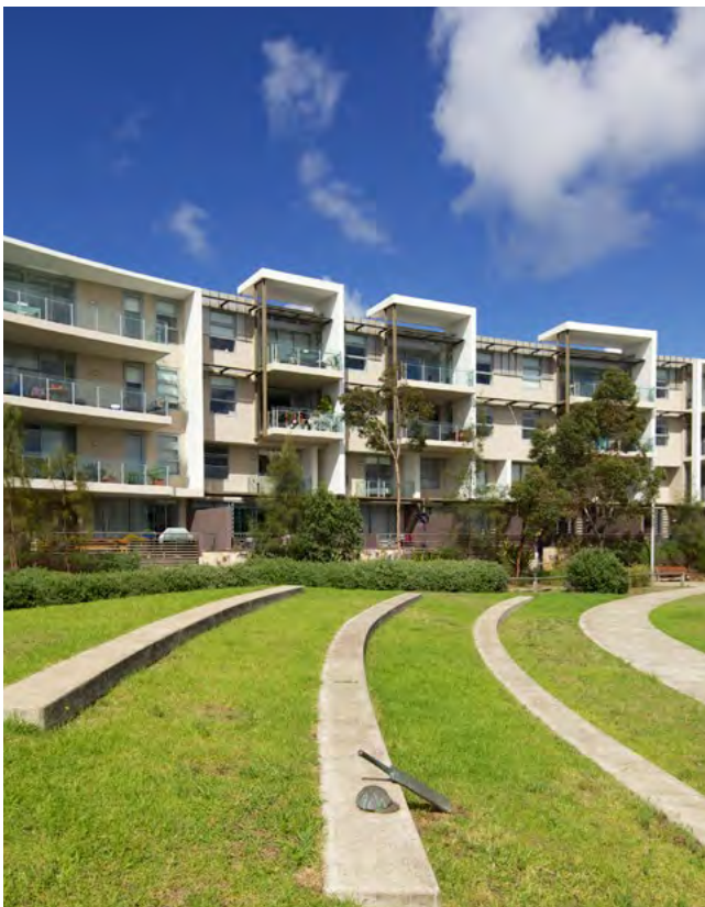
Figure 3C.6 This development makes use of landscaping, pathways and building entries to clearly identify the transition between public and private space
