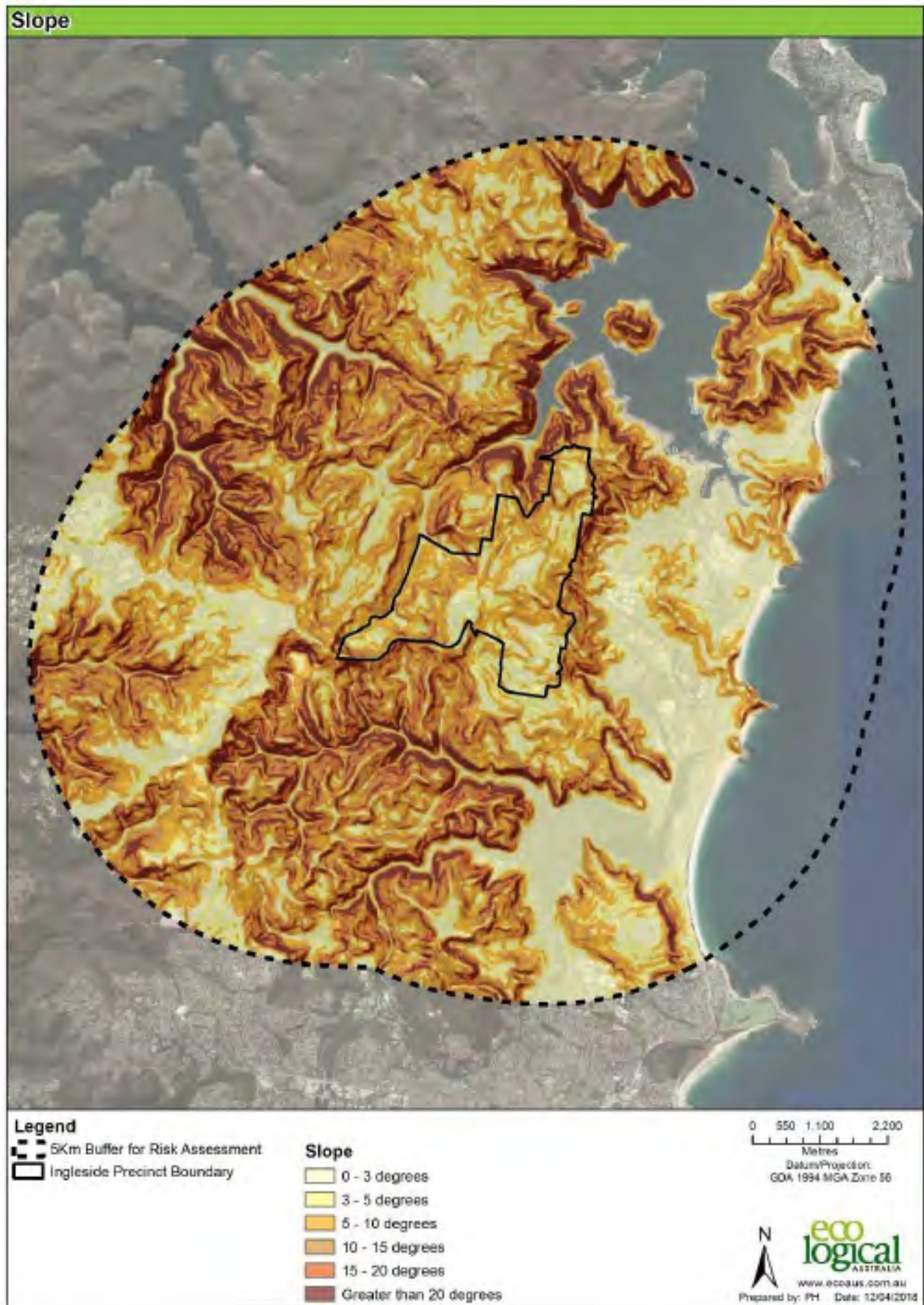
Figure 13 - Slope assessment across the study area (Source: ELA, 2018)
