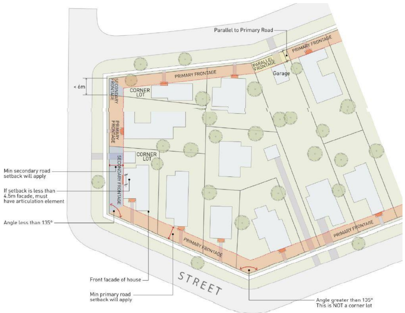
Figure 3 – Site Layout explanation for types of Road Frontages, Setbacks & Articulation Zones
