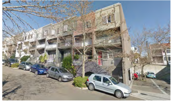
Figure 3-30 Reduce visual impact of basement entries by reducing the scale of the opening
