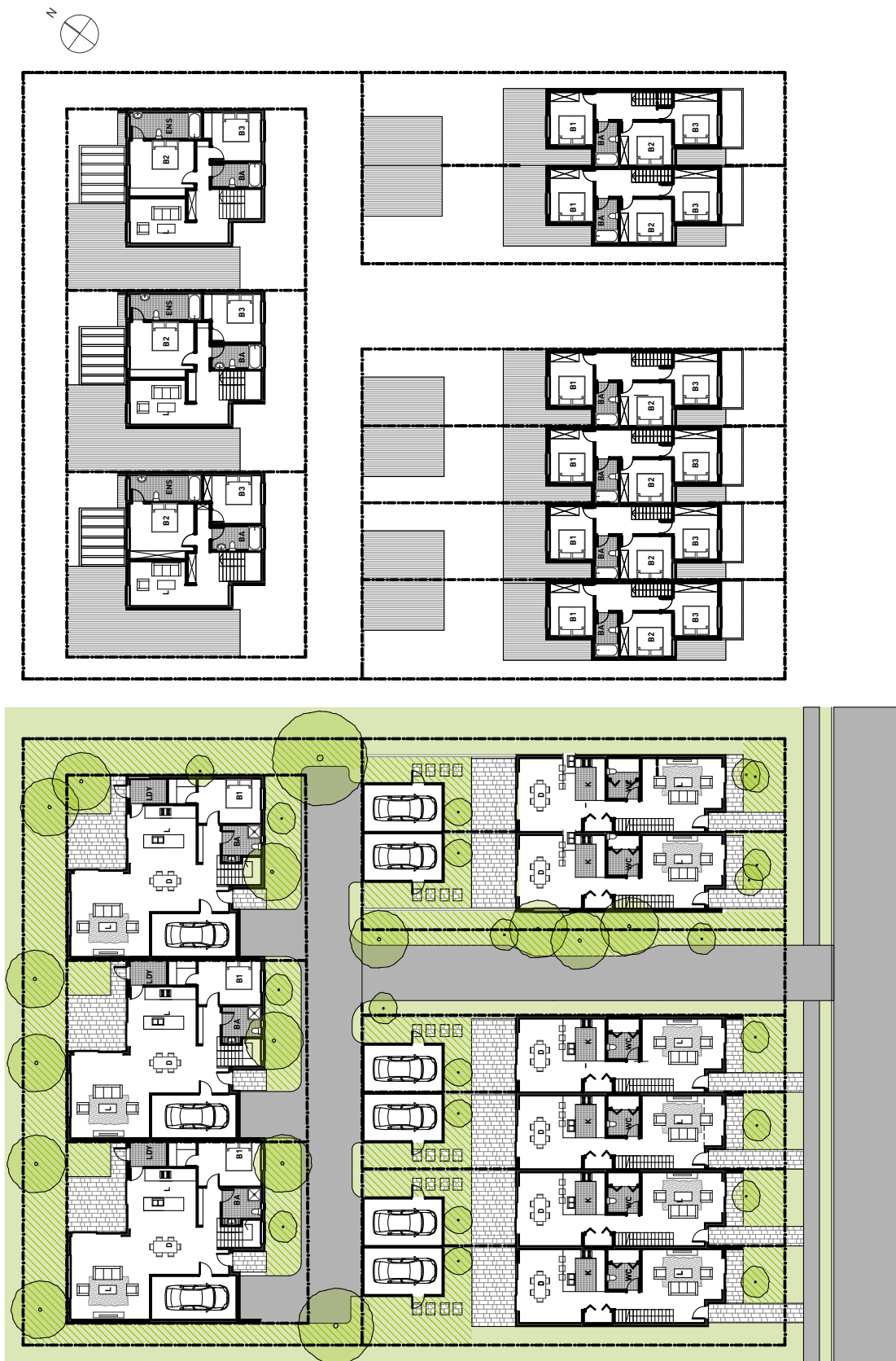
Figure 1-26 Sample plan of multi dwelling housing arranged in a 'mews' style with internal lanes
