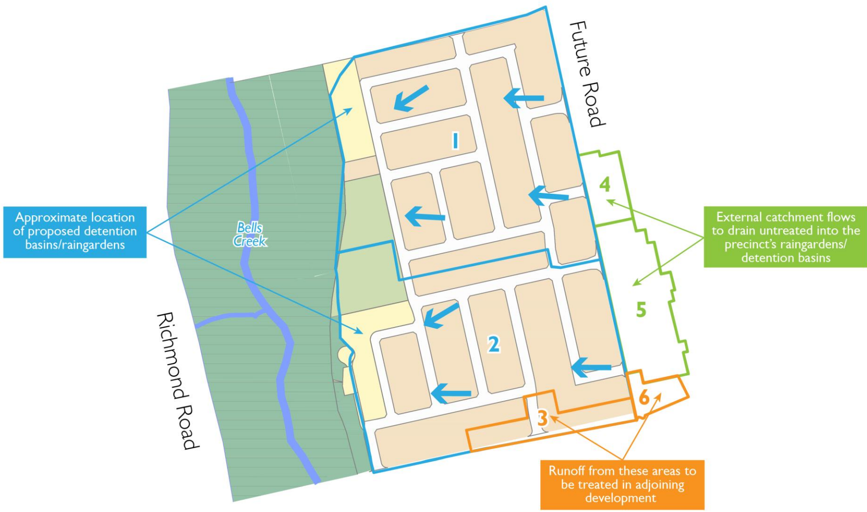
Figure 4 – Key elements of the water cycle management and ecology strategy Source: Water Quality Modelling and WSUD Assessment for Rezoning Application, Hyder (March 2014), modified by Mecone
