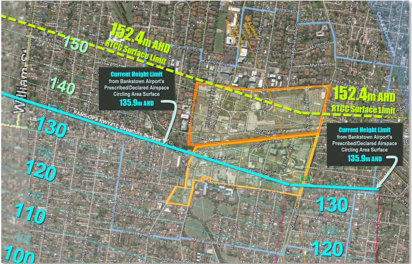
Figure 8-2: PANS-OPS Departure Surfaces Combined with the RTCC MVA Height Limit of 152.4m AHD
