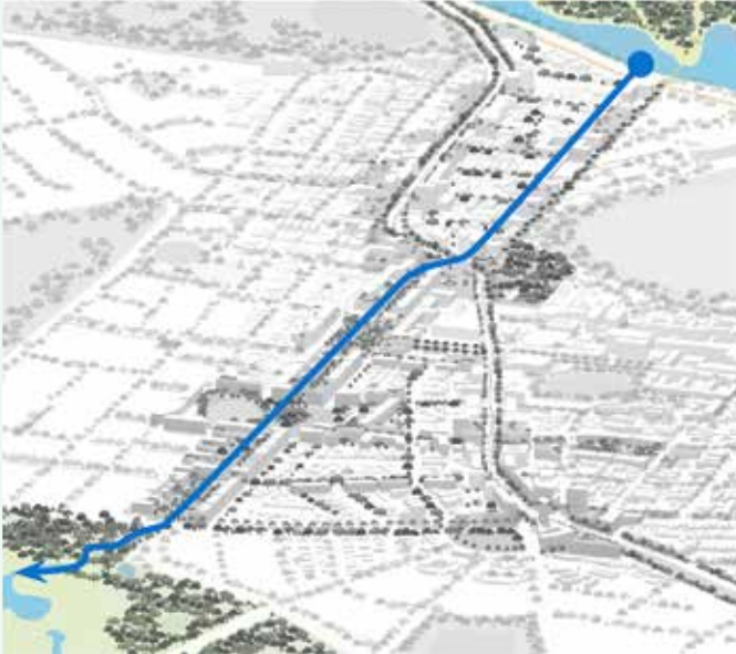
— Stormwater harvesting – rejoin ponds and wetlands
