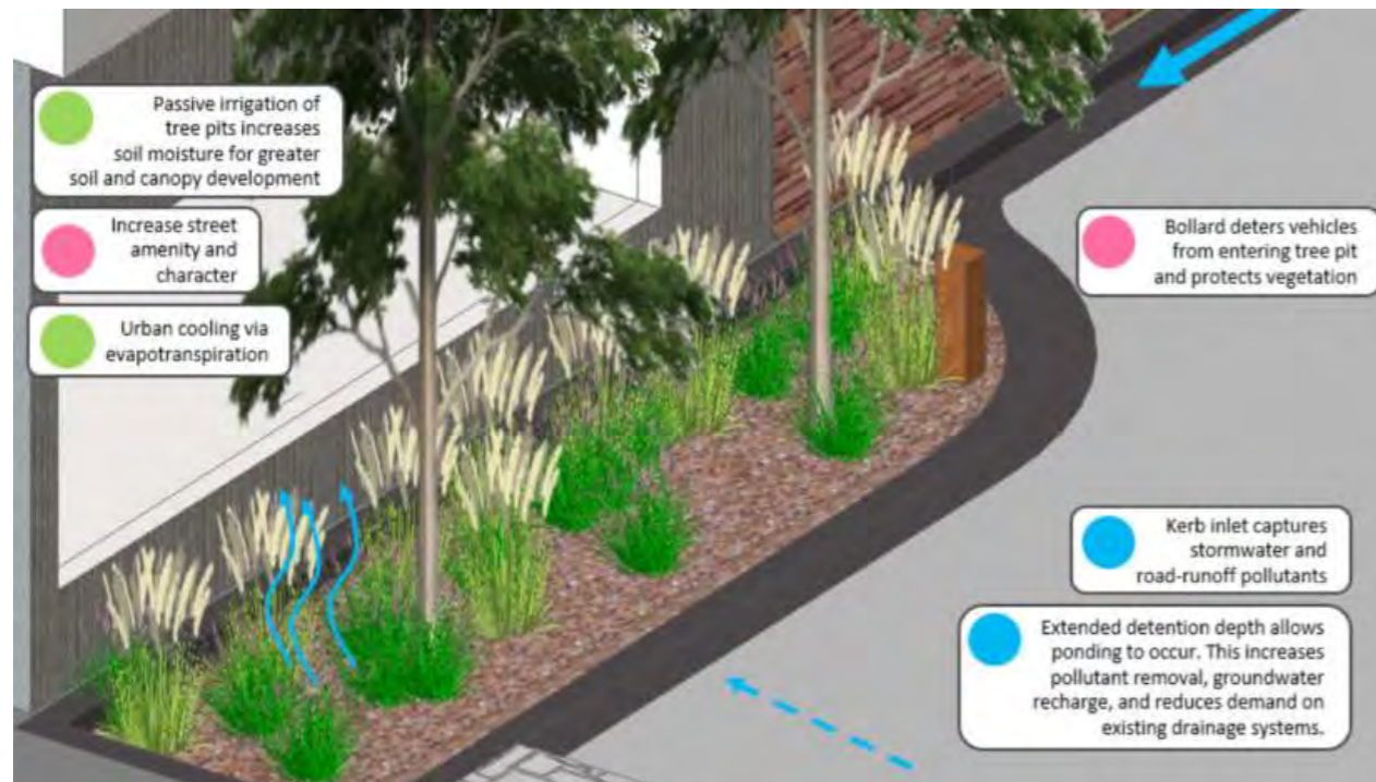
Graphic showing raingarden with trees. Source City of Yarra Embedding Green Infrastructure Guidelines
