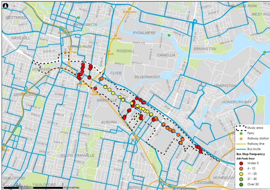
Figure 3.3: AM Peak Hour Frequency of Bus Services in the Granville – Auburn Study Area
