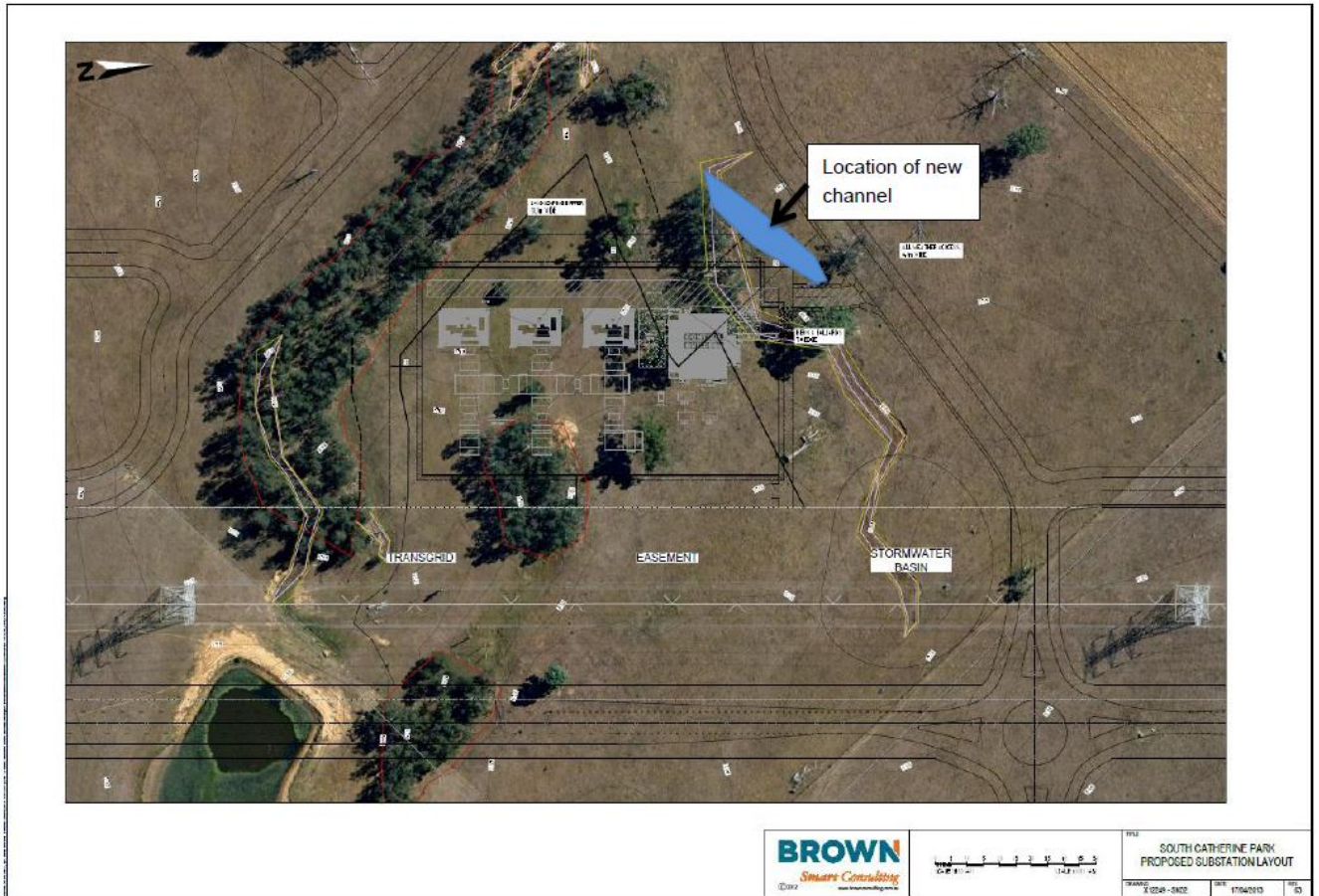
Figure 2. Substation overlaid with aerial photo. The substation footprint is the inner black line. The outer black line represents the vegetated buffer
