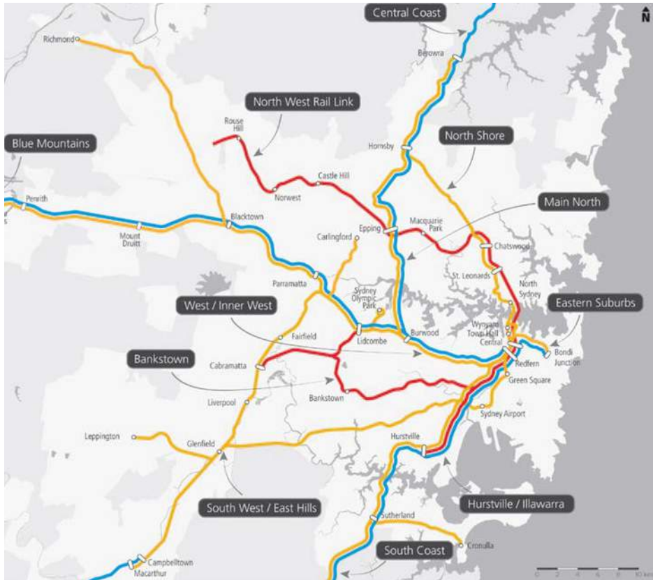
Figure 8: Sydney's Rail Future - Three-tiered System Source: Sydney's Rail Future: Modernising Sydney's Trains — Rapid transit Network (Single Deck) — Suburban Network (Double Deck) — InterCity (Double Deck) and Regional Diesel
