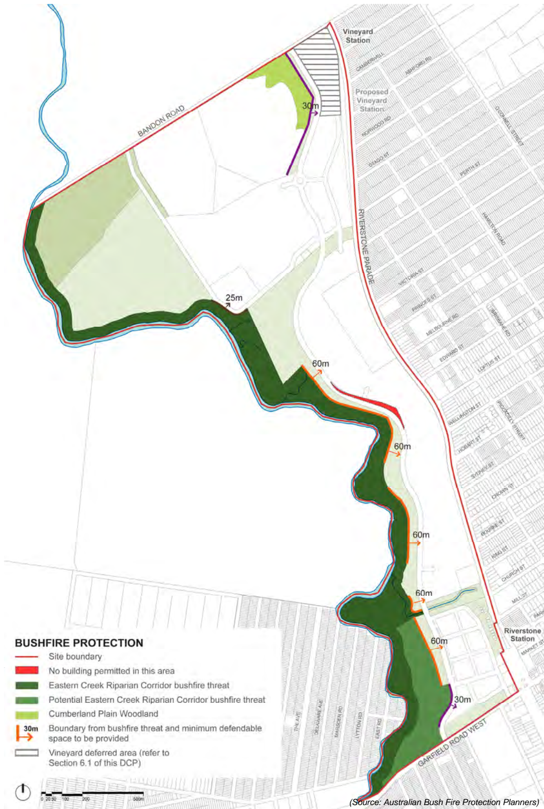
Figure 27: Defendable space for bush fire protection
