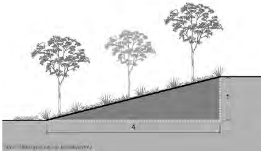
Figure 22: Indicative cross section of 1:4 embankment batter
