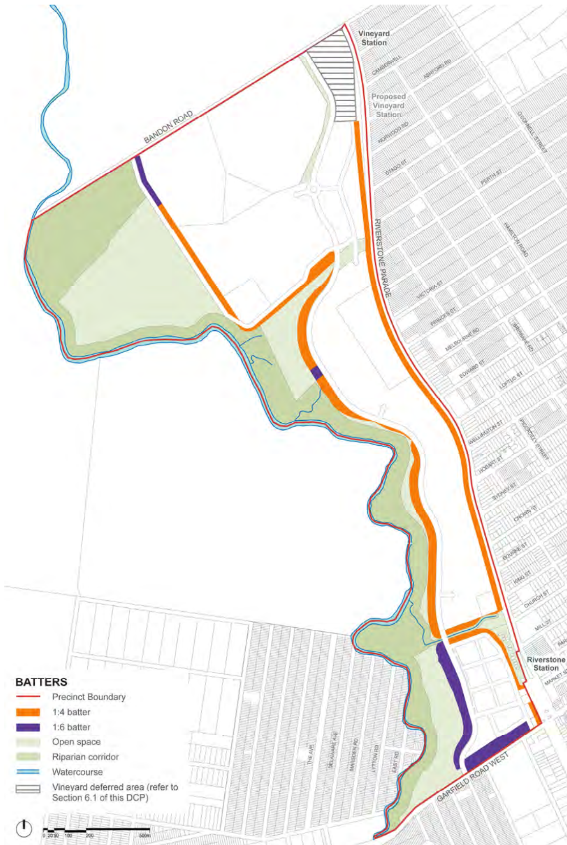
Figure 21: Location of embankment batters
