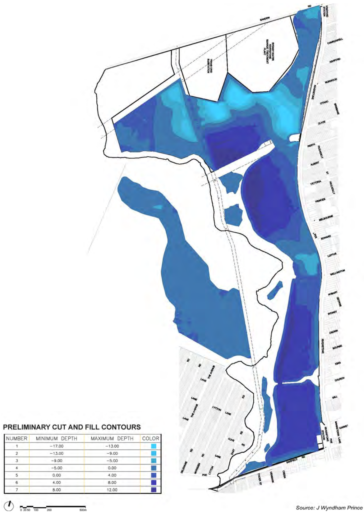
Figure C4: Preliminary Cut and Fill contours
