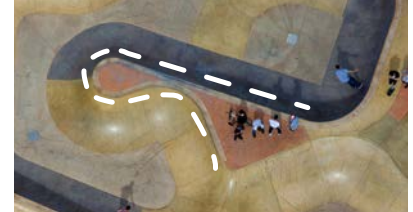
Peninsulas. A feature that juts out into a skating area, often in the form of a raised platform or obstacle.
